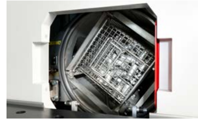
Targeted cleaning with swivelling and rotating goods carriers
