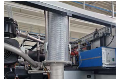
Exhaust air filtration in activated carbon module requiring no additional space
